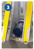
...Once your hand retracts, the light curtain automatically initiates the machine cycle...
